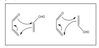
Figure 1. Hetero-Diels-alder reaction of acrolein in H<sub>2</sub>O.
